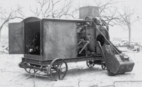
Mobile concrete mixer with lift bucket for feeding and water containers - the steel construction is riveted, about 1910 - 1930
