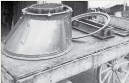
With a horse-drawn carriage a cone mould and a mould for gutters are collected around 1920
