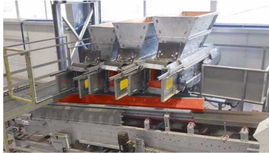
Solution Professional: Dosing of face concrete with three hoppers
