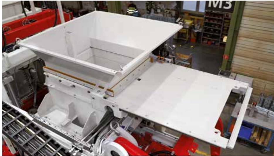
Solution Advanced: Installation of a draw plate with silo extension onto the machine hopper
