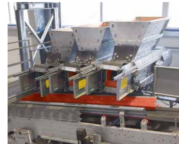
Color-Mix shuttle belt system
