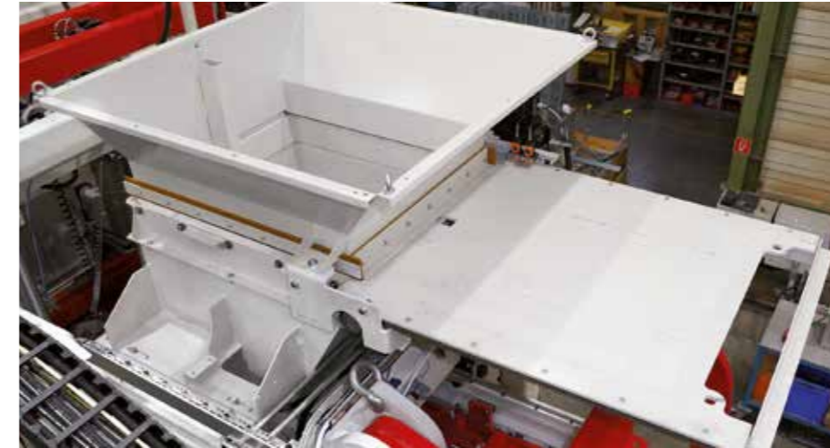
Colormix device with draw plate
