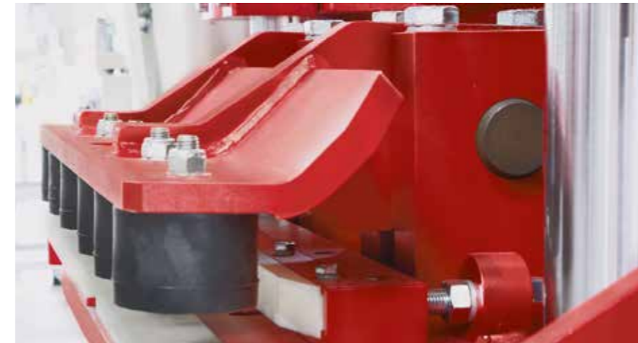
Mold side guide in the mold clamping (standard)
