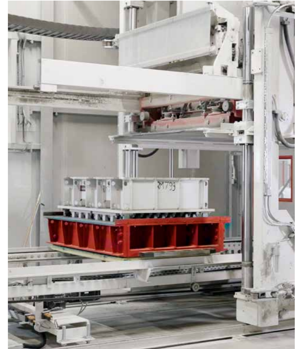
Hydraulic lifting system for quick mold change (optional)
