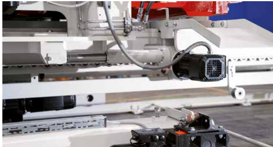
Electric horizontal table plate adjustment (optional)
