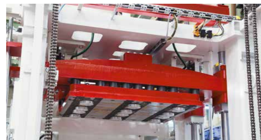
Rubberized tamper head plate (standard)
