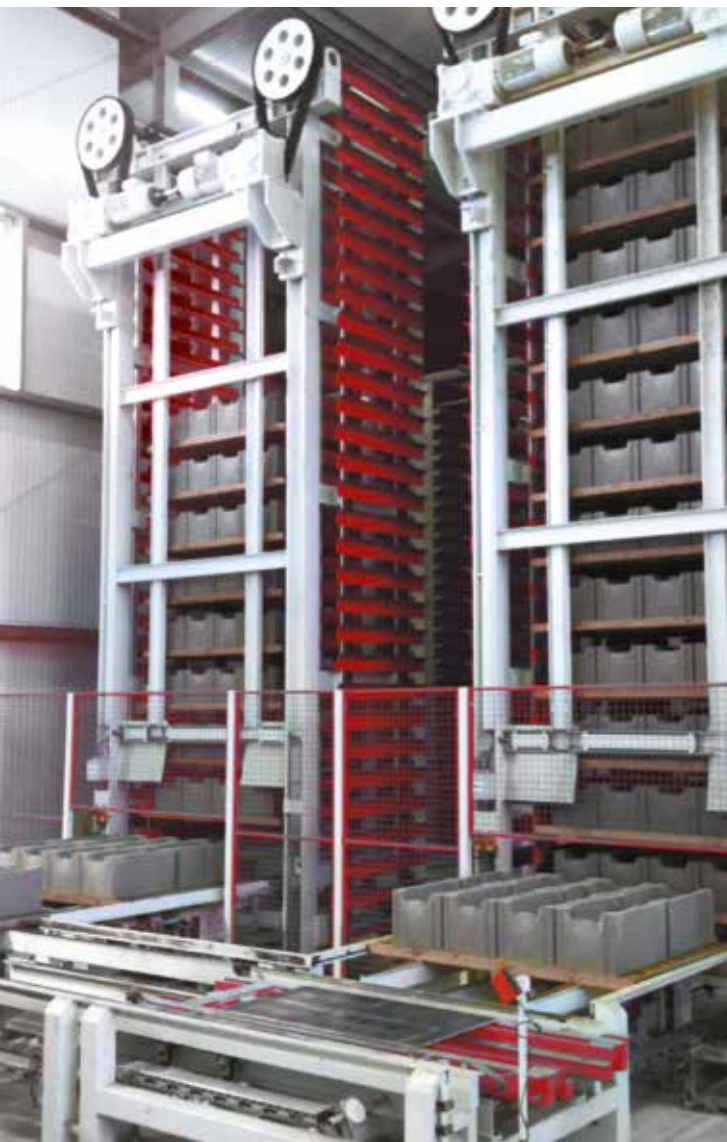
Lowerator with bypass
