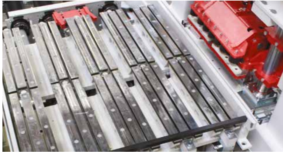
Double vibrating table and vibrator drives (optional)
