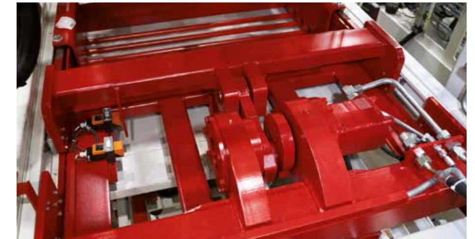
Hydraulically driven filler grid, for optimized filling of the mold and cycle time reduction
