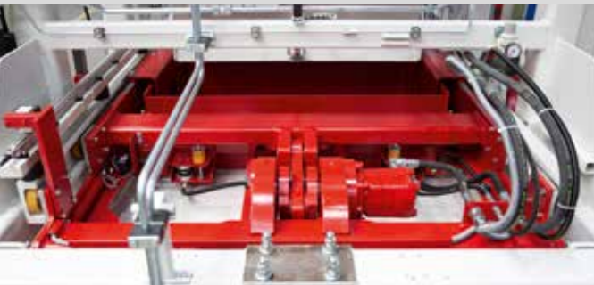
Hydraulically driven agitator, for optimal filling of the mold and cycle time reduction
