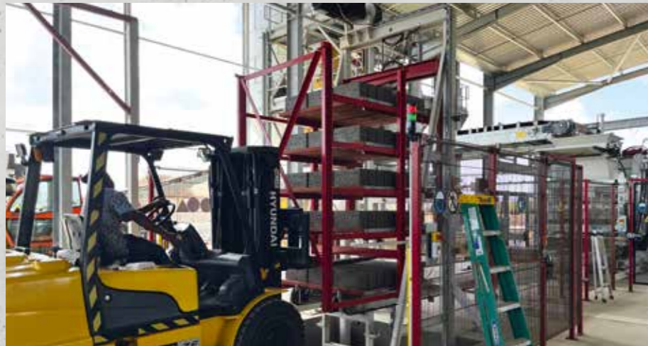
Removal of production board using forklift frames from the hoist frame
