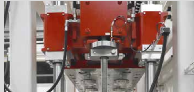
Tamper head guide with tamper head brake, for repeatable production of height-consistent concrete products with stone height stops
