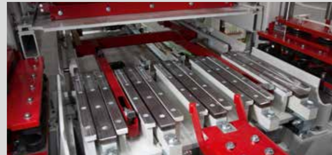
Vibrating table with 5 impact strips, for optimized compaction of high-quality concrete products
