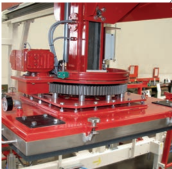
30 Universal slab transfer device-dry side
