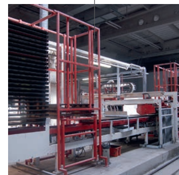
26 Flat depositing device-dry side
