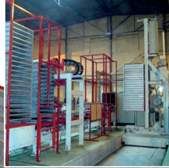
26 Flat depositing device- wet side
