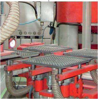
30 Green slab turning device
