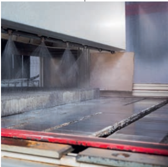
48 Special conveyor for layer-wise transport (self-cleaning)
