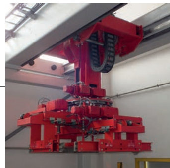
48 Cuber with electrical 4-sided-clamp and optionally with vacuum suction plate for thin slabs
