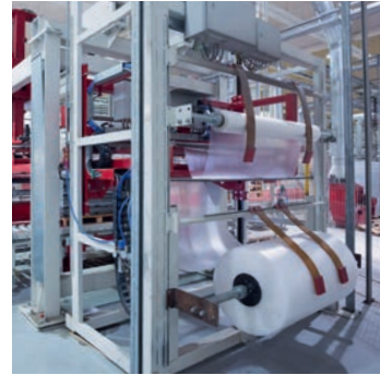
46 Intermediate layer dispenser with cover foil feeder
