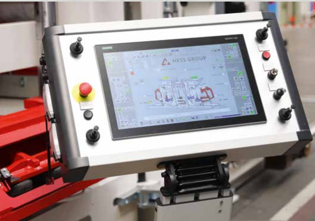
Visualization of mold and tamper head control
