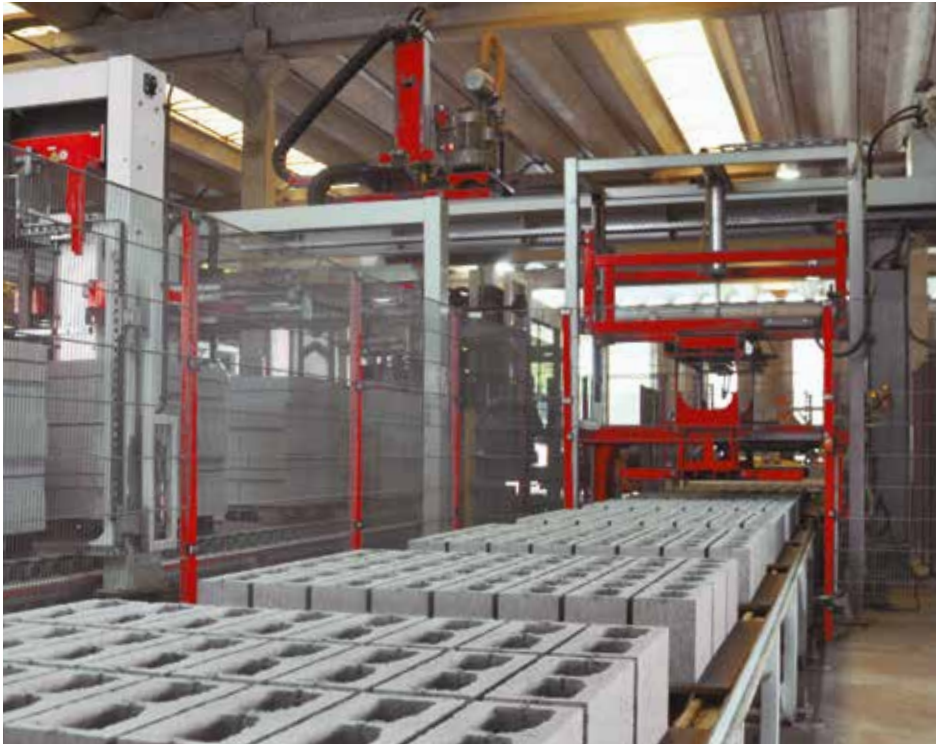
Dry side with hollow blocks
