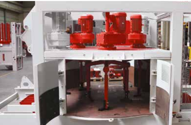
Interior view of mixer
