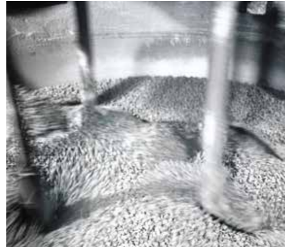
Interior view of mixer with raw materials
