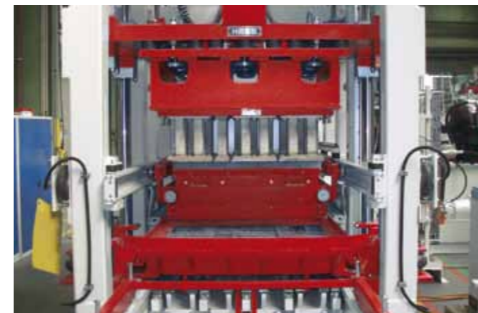
Pneumatic mold and tamper head clamping
