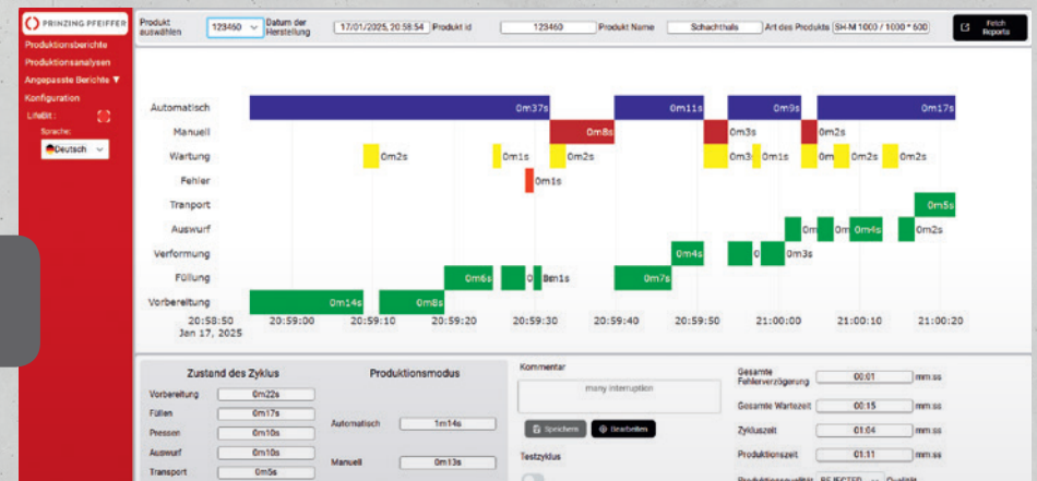
Display of machine activity (cycle times)
