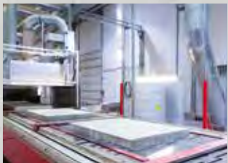
Special conveyor for layer-wise transport (self cleaning)
