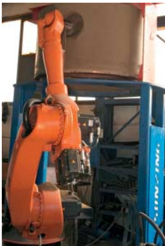
Fig. 5 Milling of connections. The manhole base section is turned as required by the inlet and outlet angles.
