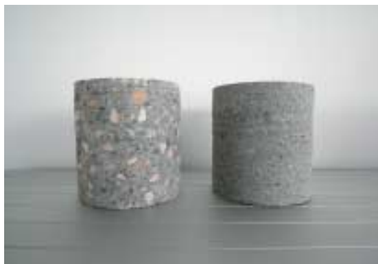
Fig. 3 Manhole base section core samples (diameter 90 mm, length 100 mm) compared: normal concrete (left), Primus base section (right).
