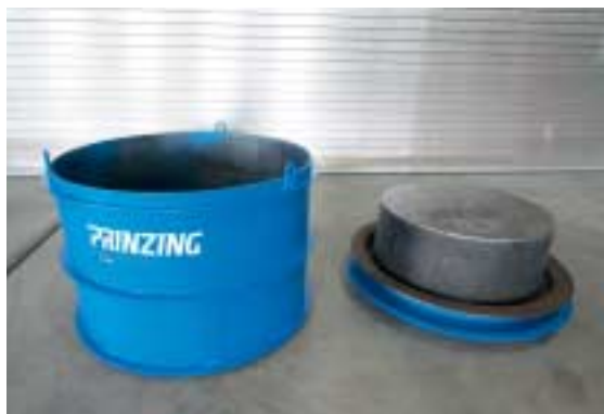
Fig. 2 The molds consist of internal support core, bottom pallets and mold cover.
